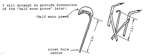
Coming off of the half moon piece to the outside of the tire is the strap which has a stud welded on the end ans is fastened to the octagon plate with a special "hand knob"made of plastic.
