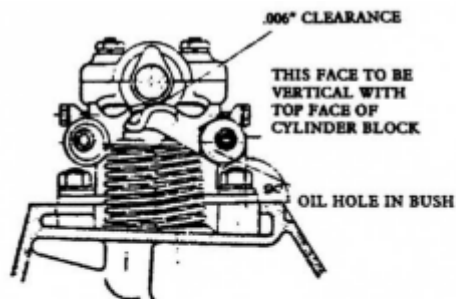
FIG. 1 SHOWING POSITION OF ECCENTRIC BUSHES FOR J. MODELS
