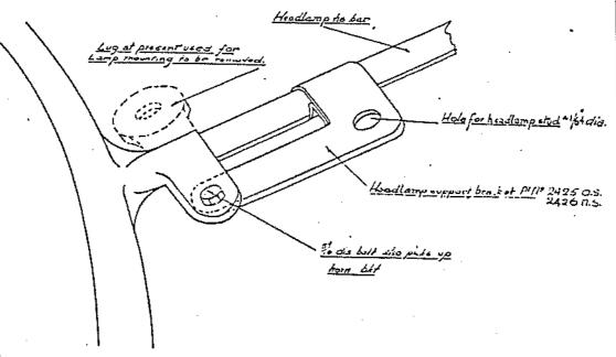
The drawing shows how this is done. The existing headlamp support lugs are cut off and filed up, the bare patch so caused being touched in with cellulose.
