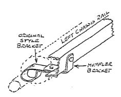
pipe was supported by a hanger on the rear dumb-iron, between the left chassis rail and the rear spring trunnion.
