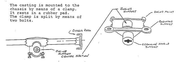
The rubber pad has a top half and a bottom half. Both pieces are identical. The pad is 1/16 inch thick and slightly protudes out front and back of the clamp. The original pad had a lip on each edge.
