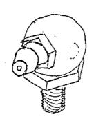
Of course there is the modern style Grease Zerk or nipple. This type has an advantage of locking onto the "grease gun" and instead of the grease coming out around the nipple, the pressure of the grease gun will force the grease into the area where you want the grease.
