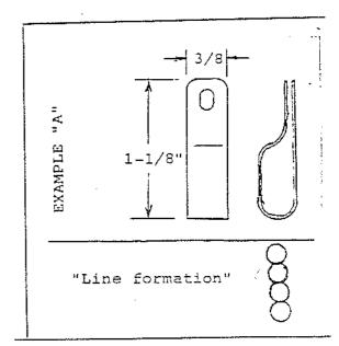
Just to the rear side of the bulk-head support the fuel line or petrol tube joins the two lubetubes and becomes a package combined in the clamping process.
