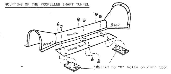
Six 1/4" bolts are required. There is some question as to how many of these bolts protude on through the floorboard and also hold the floorboard down. One authority says only the rear set is used to support the floorboard while the other says all three protrude through the floorboards. In examination of the car I tend to pick a point half way between the two authorities.
