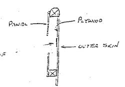
The outside of the door is covered with plywood which is covered with the exterior metal skin.
