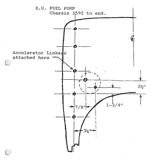
I keep on learning as one source advised me that the S.U. Fuel Pump was located in a lower position towards the end of the production. Reason -- Vaporization problems in hot weather.
