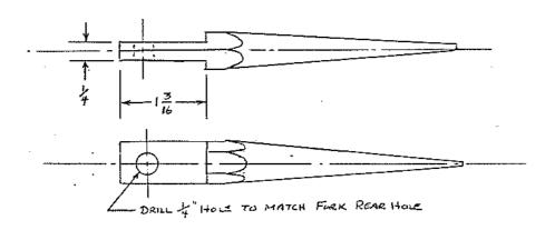
Note: the pin was ground down so the end did not stick out of the for.
