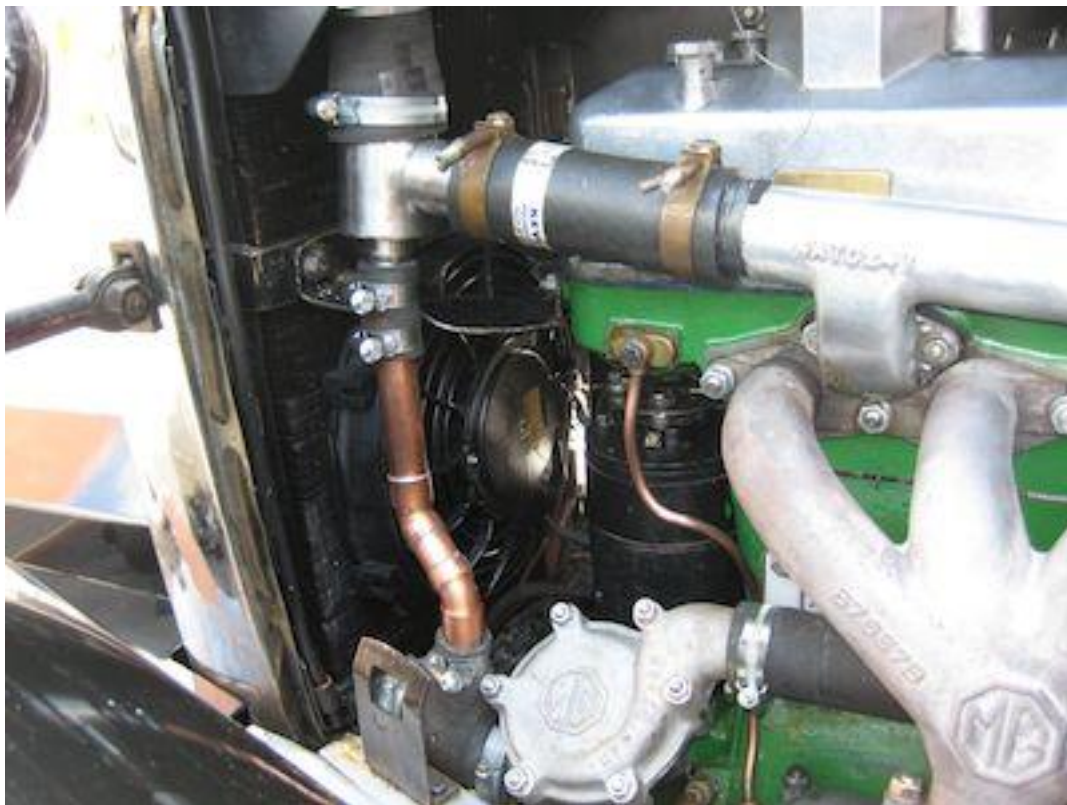
Completed installation on PB showing thermostat housing
