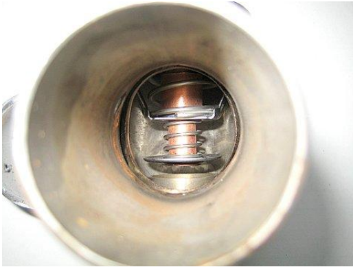
View into inlet of housing showing unseated bypass valve
