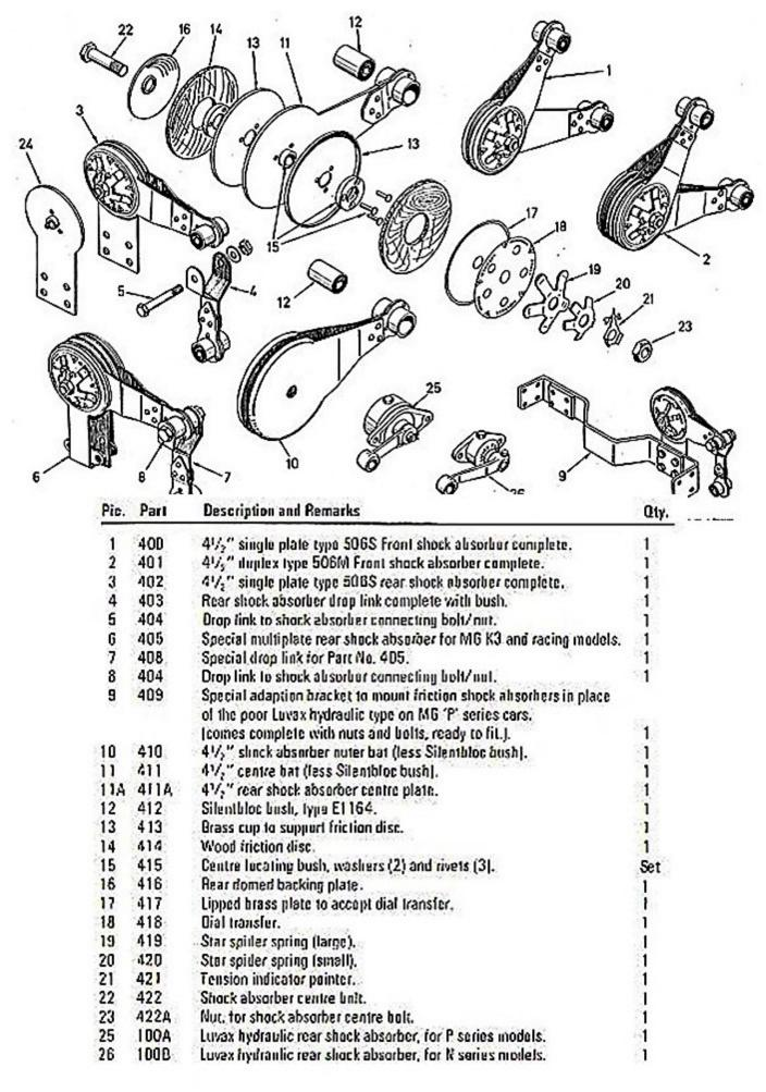
SHOCK ABSORBER TYPE 502S [Singleplate] & 502M (Multiplate) 31/4" diameter.
