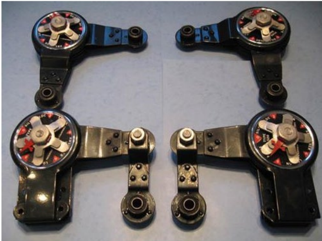
Correct 306 Front & Rear assemblies with riveted Silentbloc ends and rounded disc edge
