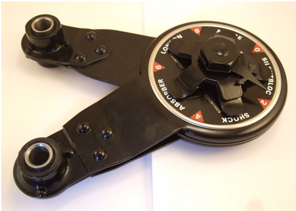
Correct 306 Assembly with riveted Silent-Bloc ends and rounded disc edge
