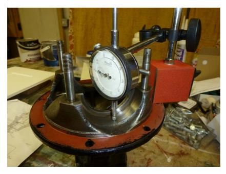
I'm sure that with a surface plate and the DTI on the magnetic base it would be possible to get a good measurement, so long as the diff assembly is carefully setup on the surface plate so the two bearing tracks are completely parallel with the surface plate.
