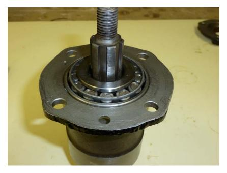
Stage 4 : Fit the Cover, the Flange and the washer and nut to finish the assembly. Only tighten the nut up finger tight to start with.
