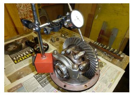
The backlash was checked at multiple points around the crown wheel. I ended up going round the crown wheel several times making measurements and adjustments.
