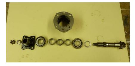
Stage 1 : Fit the two Bearing outers into the pinion carrier.
