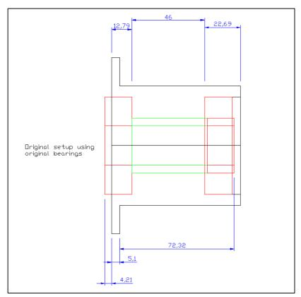
In order to maintain the same position of the pinion gear, and the flange, I felt the important measurements were the 4.21mm from the carrier flange to the bearing, and the 72.32mm from the other side of the flange to the bearing.
