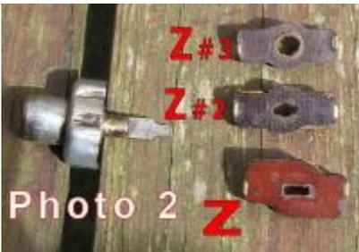
The rotor insulator - **Photo 2** - develops a round hole 'Z#3' in the Tufnol rotor insulator holder for the small brass contact plate shown at the bottom of **Photo 3**.
