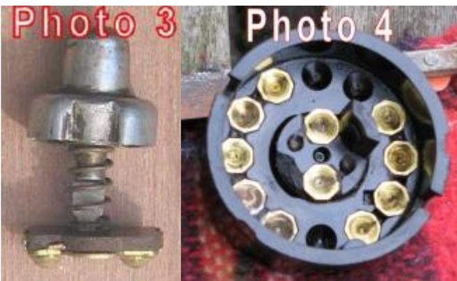
One, or both the extended lugs are broken off by enthusiastic key/screwdriver turning.....**Photo 4**.
