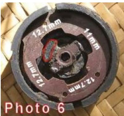
*Photo 6.* The face plate (RP in the diagram) has three lugs.
