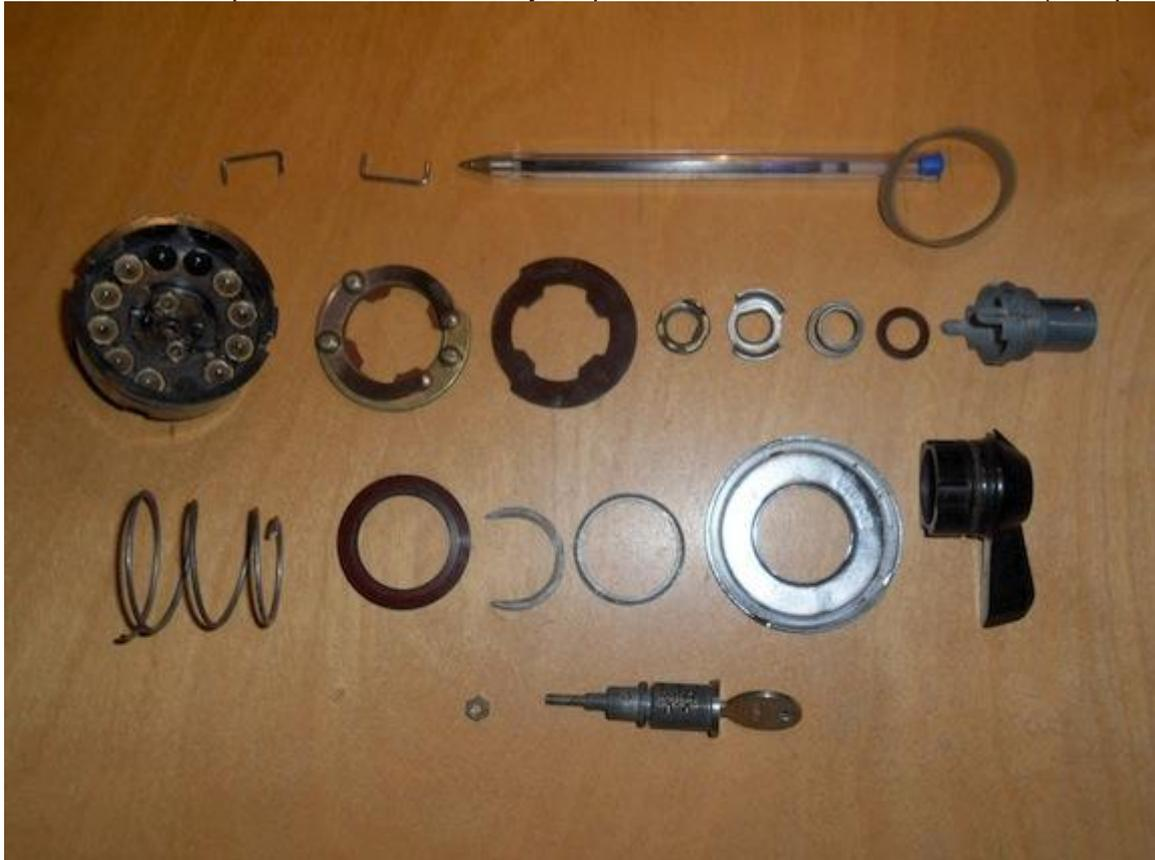
**Photo 1 – Take care in disassembling the switch!**
