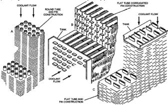
Also, higher coolant flow velocities, aided by a water pump, which promotes more turbulent flow against the tube walls which in turn enhances heat transfer into the metal 'tubes'.
