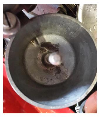
Ethanol blended fuel causes both these types of corrosion. The corrosion in my float chamber *(above pic)* was around the steel bolt connected to the aluminium body, suggesting it is galvanic corrosion. There is little information on the protection offered by the additives against galvanic corrosion and is something I will investigate further this winter.
