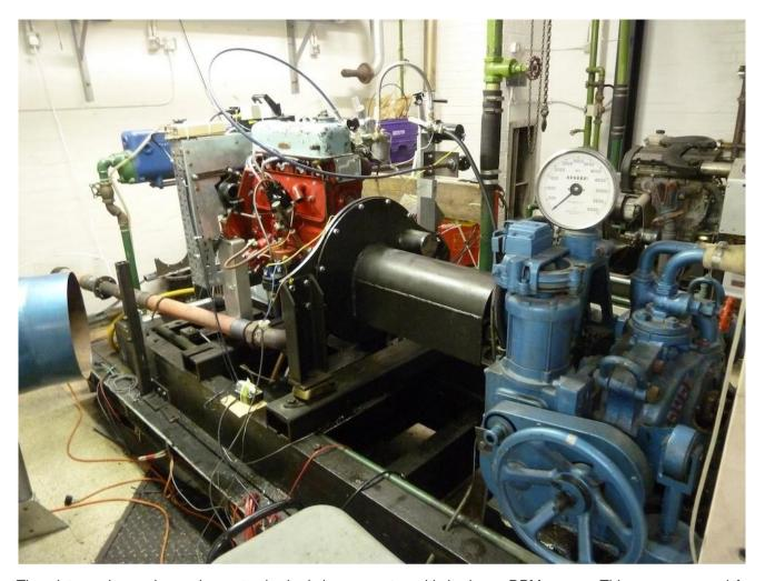
The picture above shows the water braked dynamometer with its large RPM gauge. This was managed from the control room where the gas analyser and various other readouts were located. As the pictures show, there is a lot more you can do with an engine installed in a proper test cell than you can with a rolling road.
