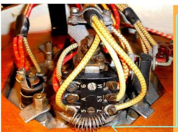
This is the resistance winding, which bridges terminal 5 and 7, so that when the switch is in position "CHARGE OFF" the dynamo-output is reduced.
