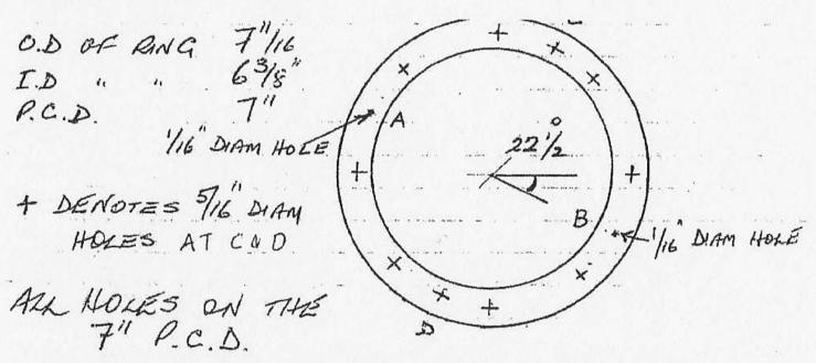
When the check has been made on the diff casing, fix the guide ring to one face of the banjo casing with two 5/16" short bolts and drill a pilot hole through each 1/16"guide hole (A&B),
